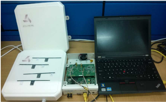
Fig. 2. Our testbed with a GNURadio/USRP2 platform and 4 WISP tags.
