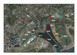
Fig. 1. Locations of deployed wind sensors on and around an urban reservoir in Singapore.
