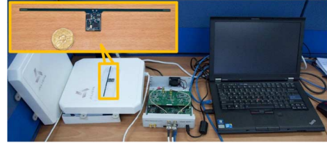
Fig. 5. Testbed: Two circular antennas are mounted to the USRP N210 software defined radio. The USRP N210 is connected via GigE to a laptop, which acts as an RFID reader. The reader interrogates WISP RFID tags.
