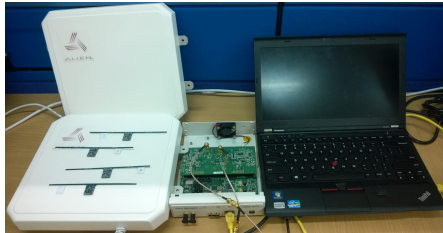
Fig. 2. Our testbed with a GNURadio/USRP2 platform and 4 WISP tags.
