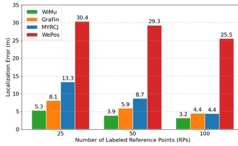
Figure 3: Localization error with different amount of labeled RPs.
