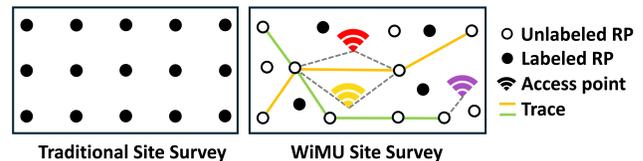
Figure 1: Comparison between traditional and WiMU site survey settings
